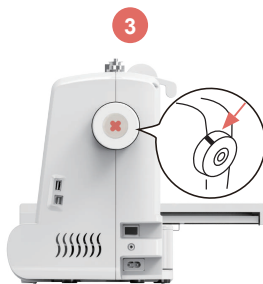
Reset the handwheel to ensure the needle is in the highest point
